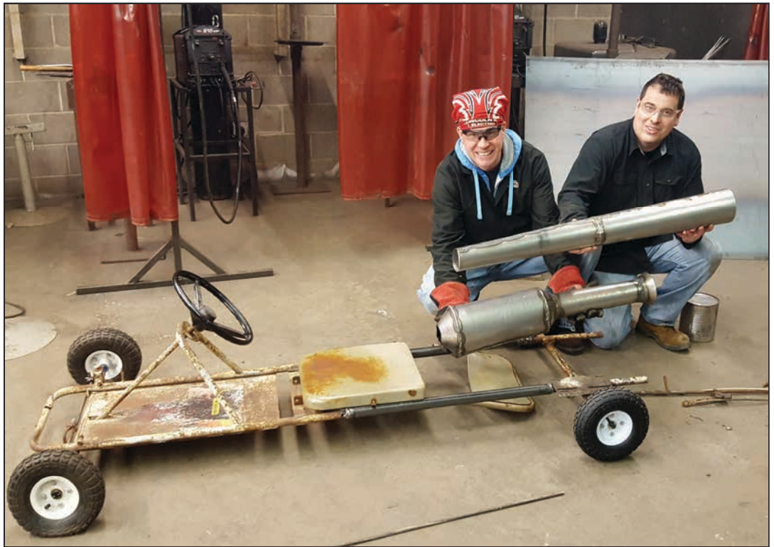
Above, Jason Kern, left, and John Stephenson built a go-kart with a pulse jet engine during their Artistic Welding Class. At right, is a bench they constructed from a truck tailgate.
